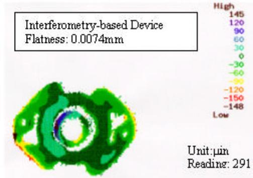
The part with a recess was later measured by another grazing-incidence interferometric device owned by a major automotive part supplier. As shown in the picture (below), the interferometric device did not only fail to detect the recess, but also created its own version of the surface (as a protrusion). Again, the reading (0.0069 mm) is not even close to the amount of recess (missed by 7 folds).
